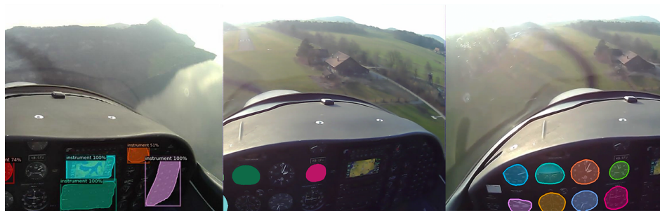
Figure 1: Flight instrument segmentation using Detectron2 (left), SAM 2 (middle), and SAM3 (right) in an Aquila AT01 aircraft.
