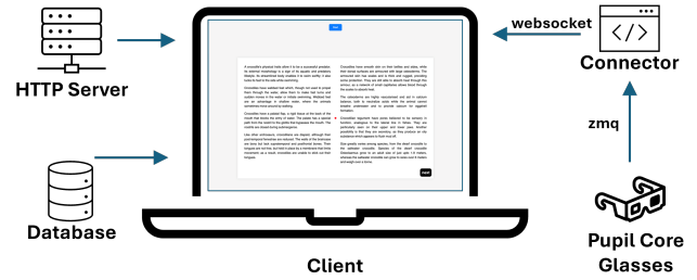
Figure 2: In our system, a Pupil Core mobile eye tracker provides real-time data via a ZMQ-socket, a pipeline prepares the data and propagates it via a Websocket, and an HTTP Server handles the serving of the client content. The client application receives the data and dynamically changes the displayed content from a database as needed.
