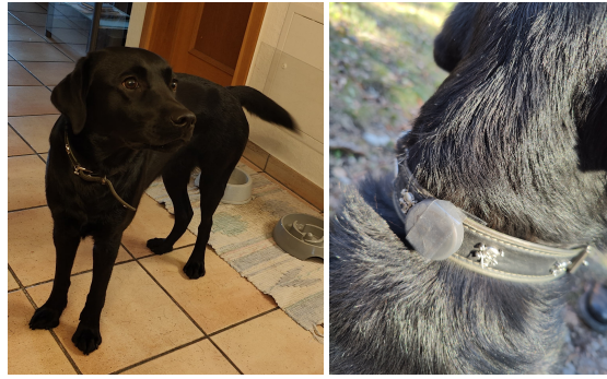
(a) Our test subject Aura (b) The Puck.js attached to the dog collar
